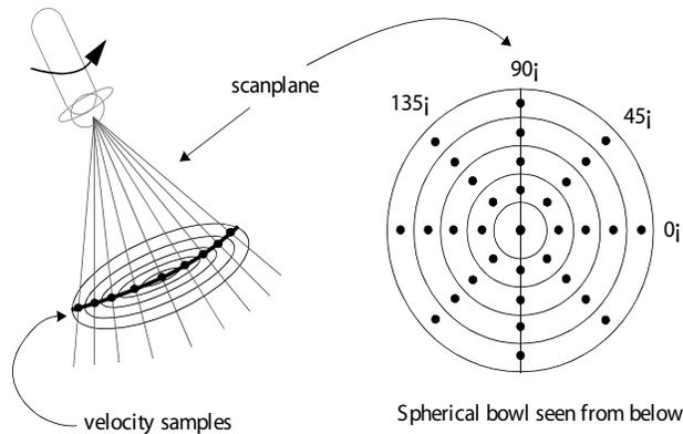
**Fig. (2).** Drawing illustrating one scan plane obtained with an ultrasound probe (left), and the 4 scan planes that are combined to obtain the spherical surface. Each dot has a corresponding surface patch.
