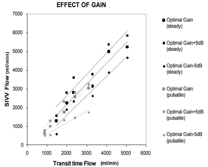
**Fig. (4).** XY plot of Transit-time vs SIVV flow for each gain setting. Steady state (black symbols) and pulsatile (grey symbols) flows. See Table 2 for regression equations.
