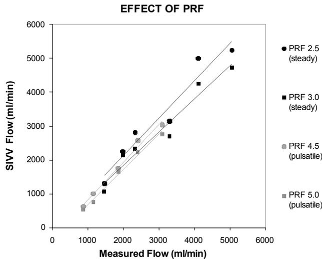
**Fig. (3).** XY plot of Measured vs SIVV flow for each PRF setting. Steady state (black symbols) and pulsatile (grey symbols) flows. See Table 1 for regression equations.
