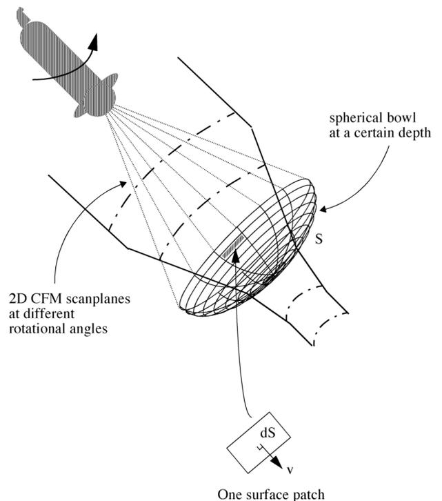
**Fig. (1).** Diagram showing the spherical control surface covering the flow area.  $S$  is the surface at a given depth, which is composed of many surface patches,  $dS$ , shown magnified with a corresponding velocity sample,  $v$ . The dotted lines correspond to the scanplanes used.
