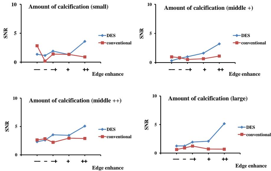
**Fig. (3).** Effect on SNR from a difference in reconstruction filter. It can confirm that SNR value increases when use a making edge enhancing filter. In addition, a dual-energy subtraction tomosynthesis processing can confirm that SNR value becomes high without coming to calcification content by amount.
