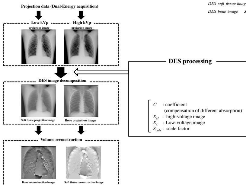
Fig. (1). Illustration of the imaging sequence and processing of dual-energy acquisition.
