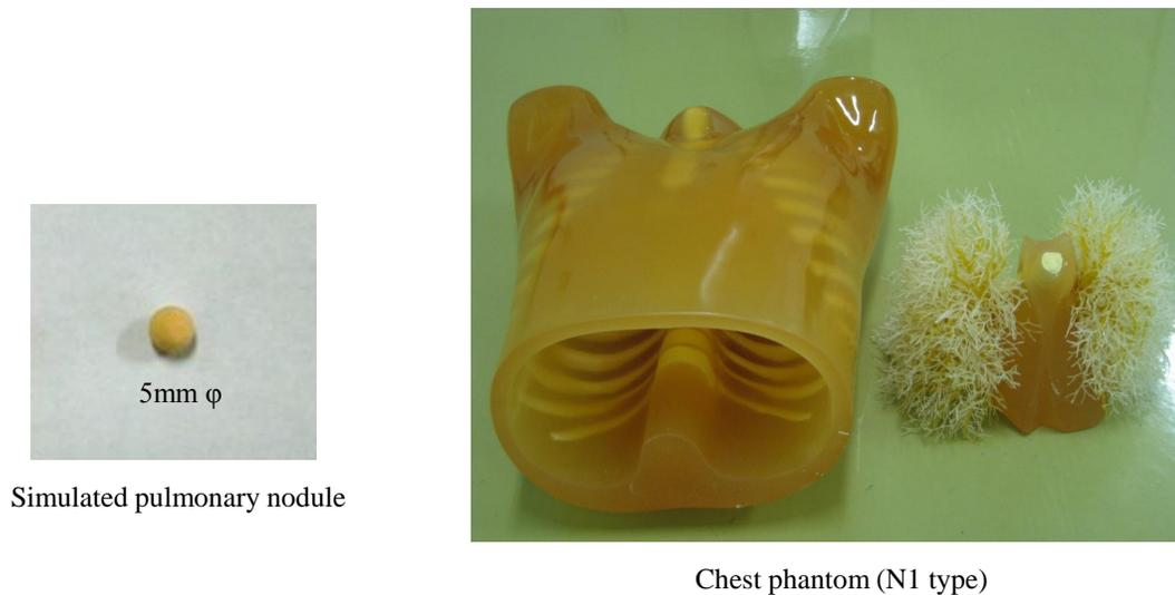
**Fig. (2).** Illustration of the chest phantom (N1 type) and simulated pulmonary nodules.
